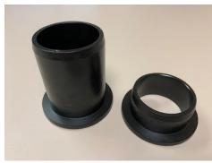
Note: Per Spec MX-5 rear shock install instructions, the rear shock alignment procedure must be followed. This example used two of the OEM spacers PT# - 9995-11-836 to achieve proper alignment of the shock though the suspensions travel under compression.
