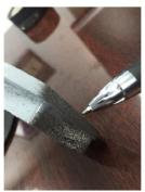
If your caliper has a wear mark or groove on it from pad burrs, you may also file the profile of the caliper to allow for proper pad fit.
