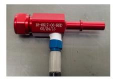
2. Unscrew the capture nut and remove the capture O-ring. Check inside the adaptor body to verify that the two O-rings inside are present, in good condition and located in the internal locating grooves.
