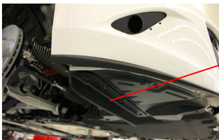
Figure 9: Plastic Angles Excluded from Ride Height Measurement
