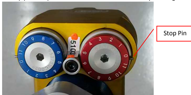
Figure 10: Damper Valve with Seal. 5 Compression, 6 Rebound Shown
