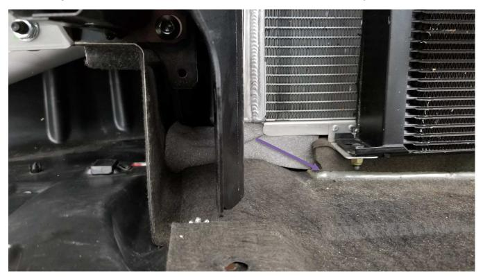
• Once Foam Is secured, Re-install Floor Panel Beneath Radiator.
