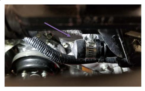
• Place 3/8 cap (Mazda Part - 0000-08-D237) on Thermostat/Water Pump Housing Nipple. Secure with Hose Clamp.
