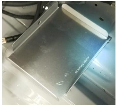
4. Install two 2-3/4" lengths of dual lock on each end of the adaptor plate, and corresponding area of the bottom of the battery.
