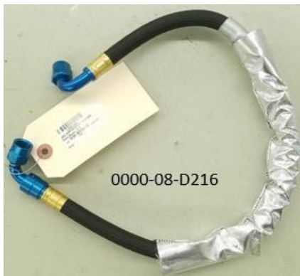
Oil Line, Diff-Cooler to Pump-ND2 0000-08-D216
