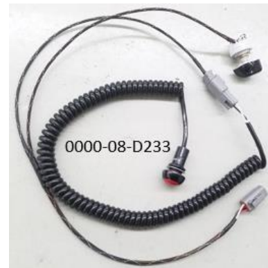
Speed Limiter, Pit Lane-ND2 0000-08-D233
