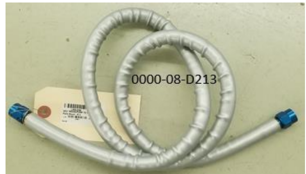
Oil Line, Trans-Pump to Housing – ND2 0000-08-D213
