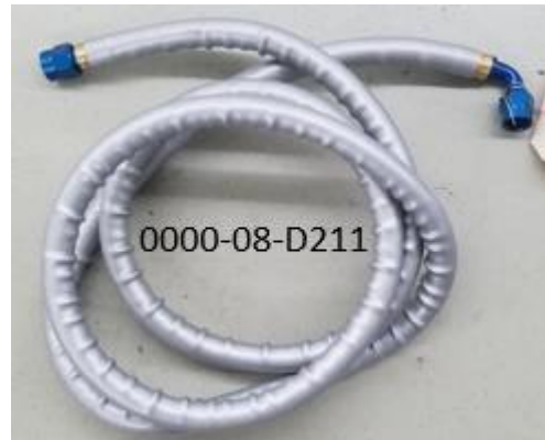
Oil Line, Trans-Filter to Cooler-ND2 0000-08-D211
