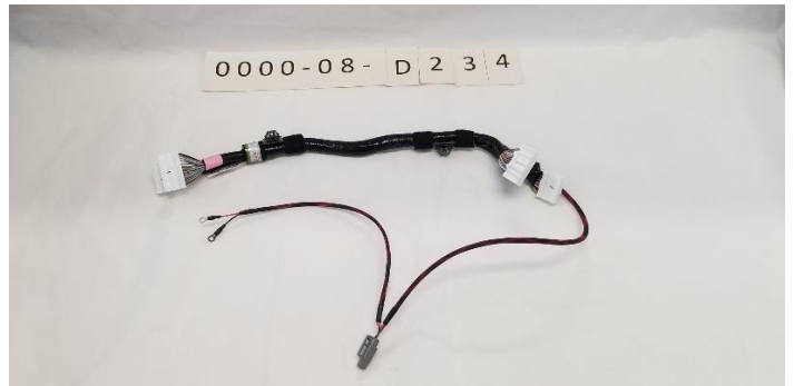
Modified start/stop wiring harness - 0000-08-D234
