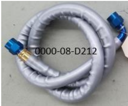
Oil Line, Trans-Cooler to Pump-ND2 0000-08-D212
