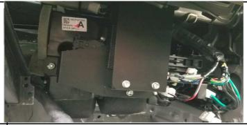
17 Remove 3 M6 Bolts to Remove ECU Capture at Bottom of Bracket and Install Bosch MS6 Cup ECU, Snap it Into Place at top of Bracket with Dual Lock and Reinstall Bottom Bracket Capture.
