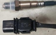
4 (new Rev 6) The Rear O2 Sensor is Not Functional and it's Connector No Longer Matches the Engine Harness. You May Tie Up Each End of the Wires Without Connecting them, or You May Remove the O2 Sensor and Replace with a Standard Exhaust Plug.
