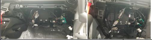
17 Route +12V, and GND Wires on ECU Adaptor Harness with Main Chassis Harness on the Left Side Transmission Tunnel near the Right Rear Damper. Final Routing and Connection for this is completed in the Aftermarket Wiring Updates section.
