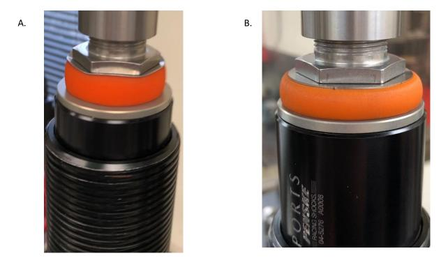
**Fig A**. Shows current shim/plate (.020" thick) deformation at .125" displacement. The deformation is not a concern because the shim is actually molding itself around the sharp edges of the nut. This is does not add risk of bump stop degradation as it continues to protect the stop from the corners of the nut.
