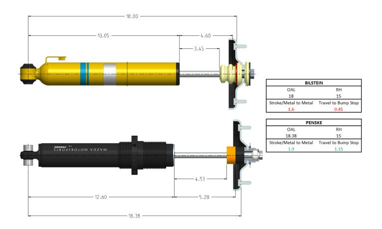
**Bump Stop Performance** - The Penske set-up uses a 70-durometer rated .750" thick stop; the Bilstein uses foam 1.5" (Est) stop. The Bilstein is a softer stop and will displace more while having less rate.
